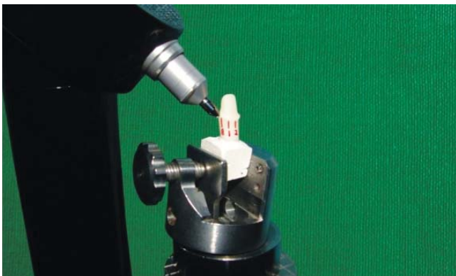
Fig.11 Scanning of master die with Contact scanner- Procera system
